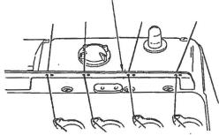
(Caution) When using an untwisted thread such as wooly nyton thread or weak thread, do not wind it round the intermediate thread guide.
