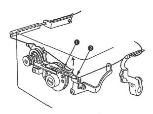
(Caution) Raise looper thread cam thread guide ① and perform threading. Return looper thread cam thread guide ① to its home position and securely fix it to retaining spring ②.
