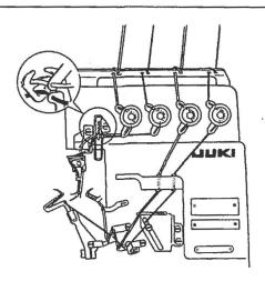
(Caution) Be sure to pass the needle thread for double chainstitch through the needle thread take-up lever.
